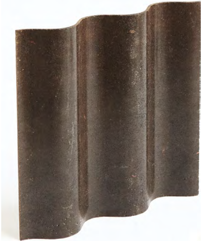
Hemp and sugarcane resin panels by Margent Farm
