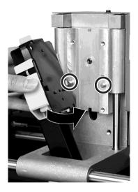
Insert the cap screws at the locations shown in the figure, and tighten them loosely using the included hexagonal wrench (size: 3 mm). After attaching all four screws in this way, tighten them securely.
