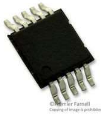
The HVSSOP package has a PowerPAD.
