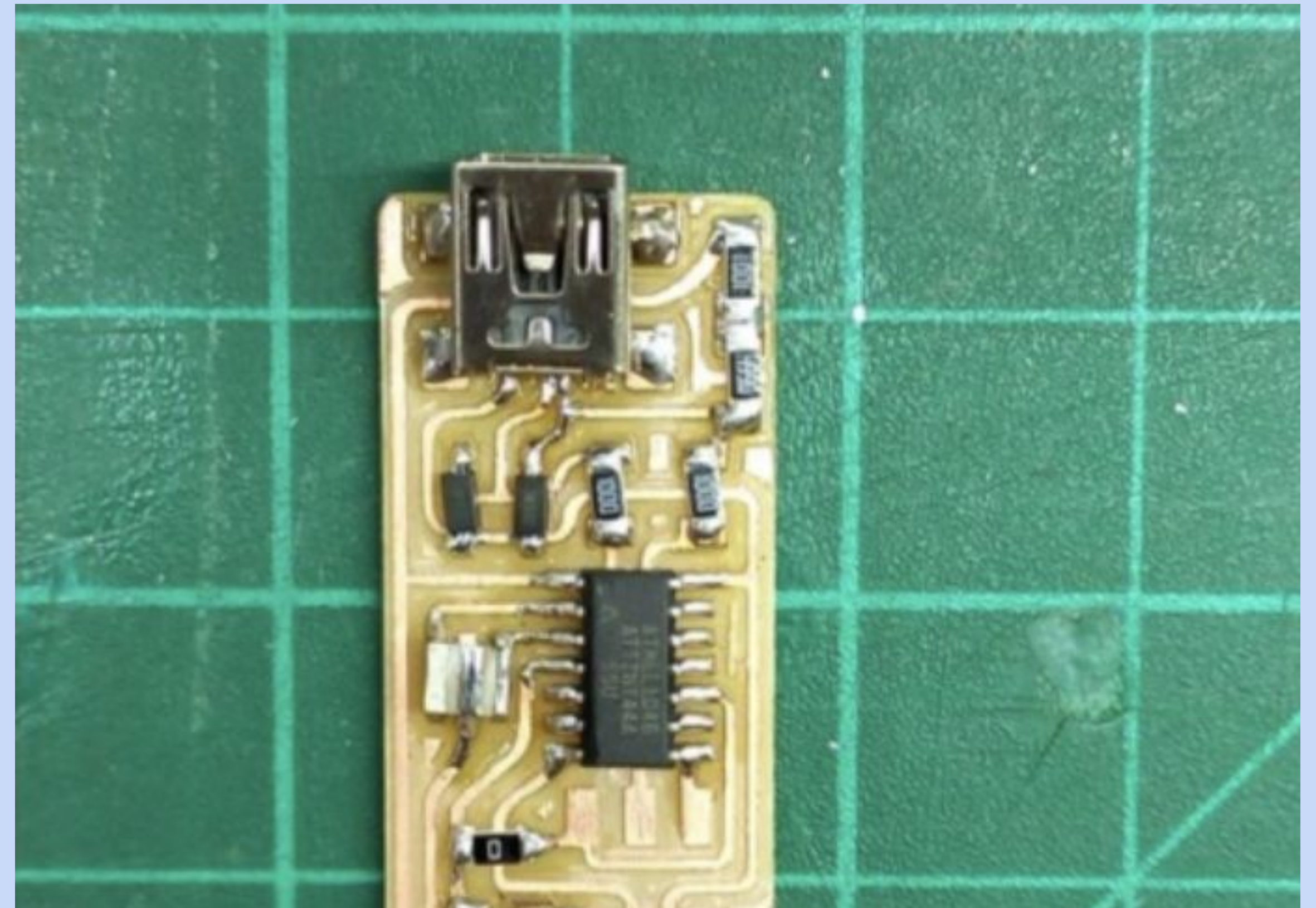
PCB with components - made by Amany - Fab Academy 2022
